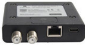
EoC MediaConverter - COAX to 1Gbps IP network
